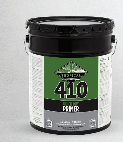
**#410 Quick Dry Primer** is an asphalt-based material used as a fast-drying bonding coat and for priming surfaces prior to the application of cold applied and hot mopped asphalt coatings, roof cements, mastics and adhesives. **#410** dries fast and is ready to use as it comes from the can. Not recommended as a stand-alone roof coating.
