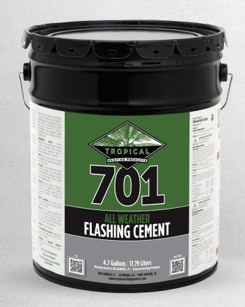
**#701 All Weather Flashing Cement** is a professional grade asphaltic base flashing cement that adheres to all surfaces wet or dry. Readily adheres to all prepared surfaces, and will not sag, slip, or mud-crack. A multipurpose flashing cement for repairing leaks, cracked spots, holes in shingles, concrete, and steel or metal roofs. Can be used on all flashings around skylights, gutters, and in all crevices. Meets and exceeds all the requirements of ASTM D 4586 and D 3409.
